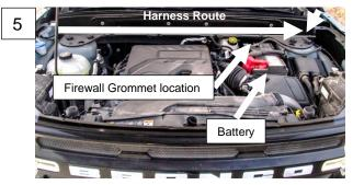
To route the switch through the firewall, the battery will need to be removed. First, remove the intake ducting from above the radiator by prying the two arrowed plastic fasteners with the trim tool.
