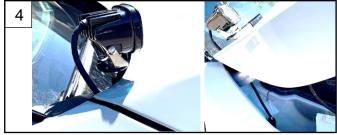
Attach harness leads to each power cords and route along the upper firewall. Use the provided wire ties to fasten the harness to the plastic inner wiper cowling.
