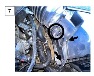
8. Loosen the circled battery clamp fasteners with the 10mm socket with the extension. Remove the battery terminals (+/-) with the 10mm socket and place them aside; black lead first. Now the battery can be slid forward and removed for the moment. Remove the arrowed firewall grommet and route the harness switch lead through. Pull enough slack in from inside the cab to reach the headlight controls.
